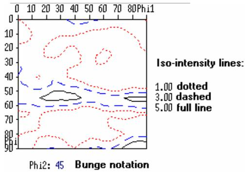
Figure 1. ODF section at  $\phi_2=45^\circ$  of 1.25%Si steel.
