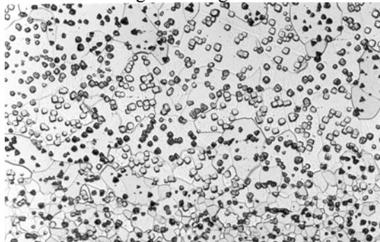
Figure 4. Etch pits show cluster of (100) fiber grains in the grain size region. Magnification 127x.
