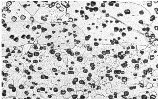
Figure 3. Etch pits show rectangles of Goss orientation in the small grain size region. Magnification 230x.
