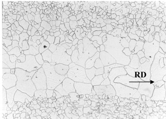
Figure 2. Section parallel to sheet surface showing cluster of large grains surrounded by clusters of small grains. Magnification 100x.
