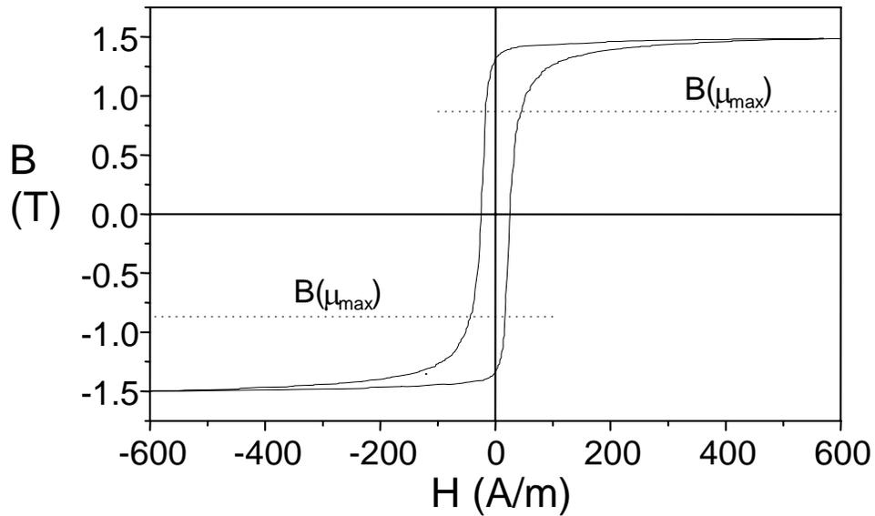
Figure 3. Hysteresis loop of the 358µm sample, rolling direction, showing the position of the maximum permeability induction.
