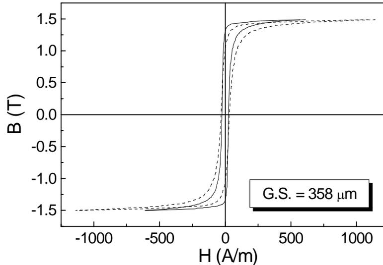
**Figure 2. Hysteresis loops of the sample with grain size of 358 $\mu\text{m}$ , measured on the rolling (full line) and transverse direction (dotted line)**
