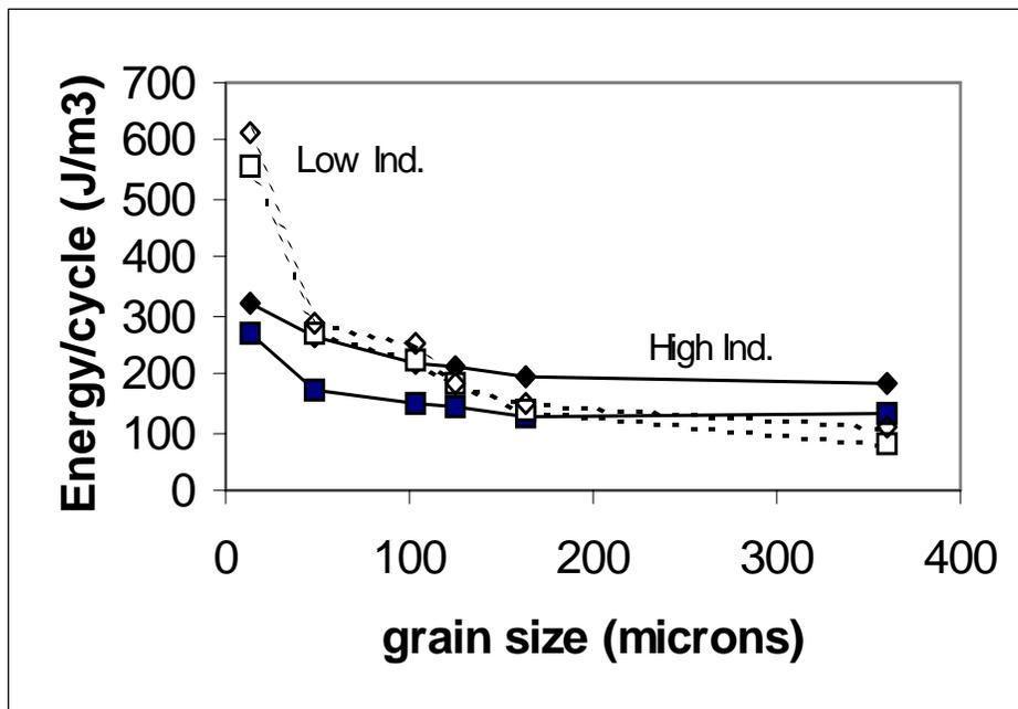
Figure 4. Effect of grain size on the Energy Loss / cycle in the Low Induction component (dotted line) and in the High Induction component (full line), measured in the Rolling direction (□) and Transverse Direction (◇).
