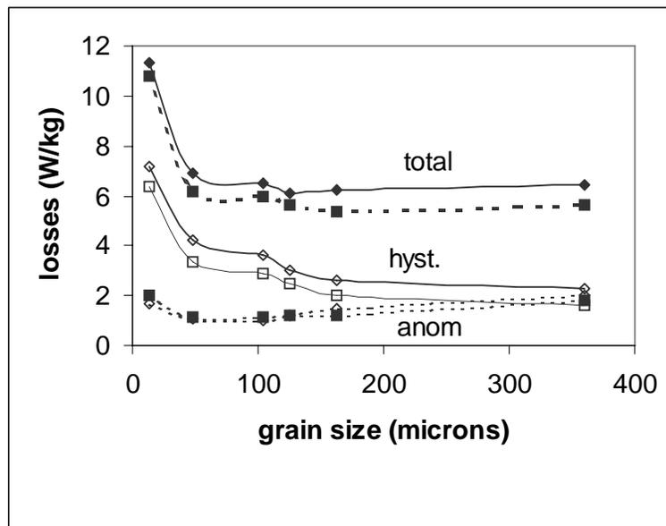
Figure 1. Effect of grain size on Total Magnetic Losses, Hysteresis Loss and Anomalous Loss at 1.5T 60Hz, measured in the Rolling direction ( $\square$ ) and Transverse Direction ( $\diamond$ ).
